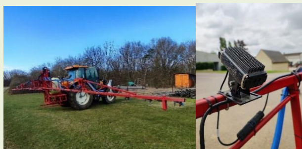
Sprayer equipped with spot spraying sensors on a farm in Saint-Hilaire-en-Woëvre (France). The sensors used are from the company CarbonBee. ©ARVALIS
